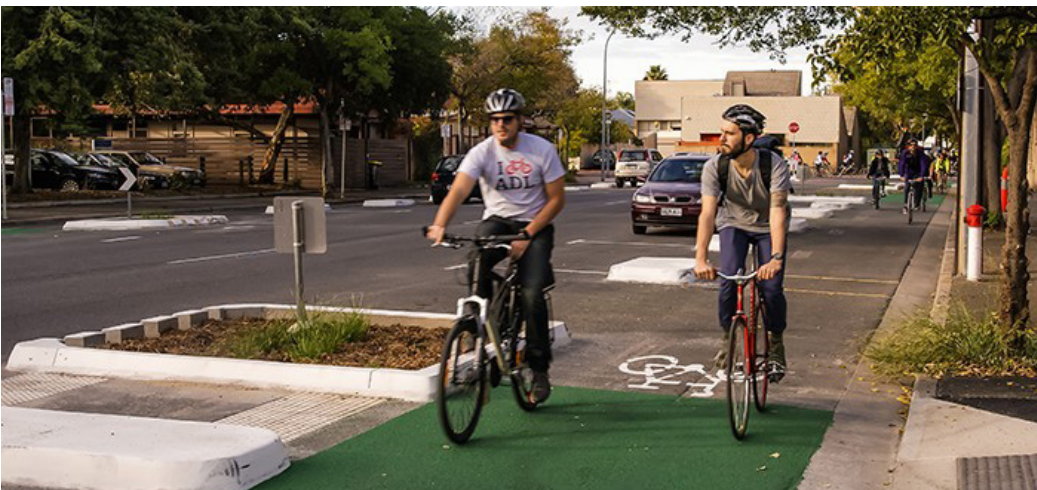
Class IV Bikeways provide exclusive separated lanes for the exclusive use of bicyclists.
